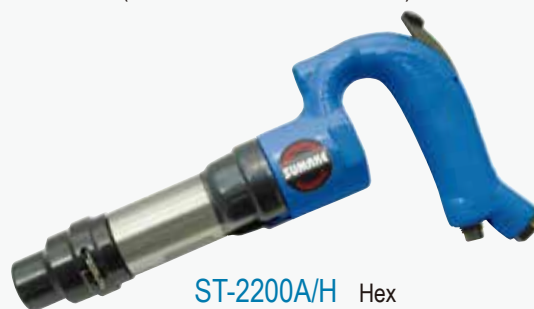
ST-2201/H(R) 1" Piston stroke (2,820 b.p.m) ST-2202/H(R) 2" Piston stroke (2,150 b.p.m) ST-2203/H(R) 3" Piston stroke (1,920 b.p.m) ST-2204/H(R) 4" Piston stroke (1,500 b.p.m) Air chipping hammer (H: hex shank, R: round shank)
