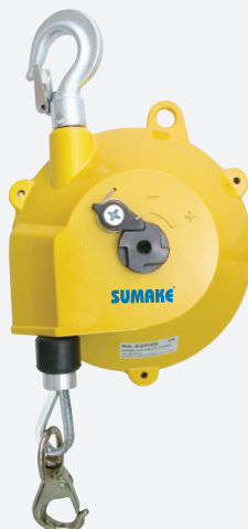
SA-22030 (1.5-3.0kgs) SA-22050 (3.0-5.0kgs) SA-22070 (5.0-7.0kgs) Spring balancer
